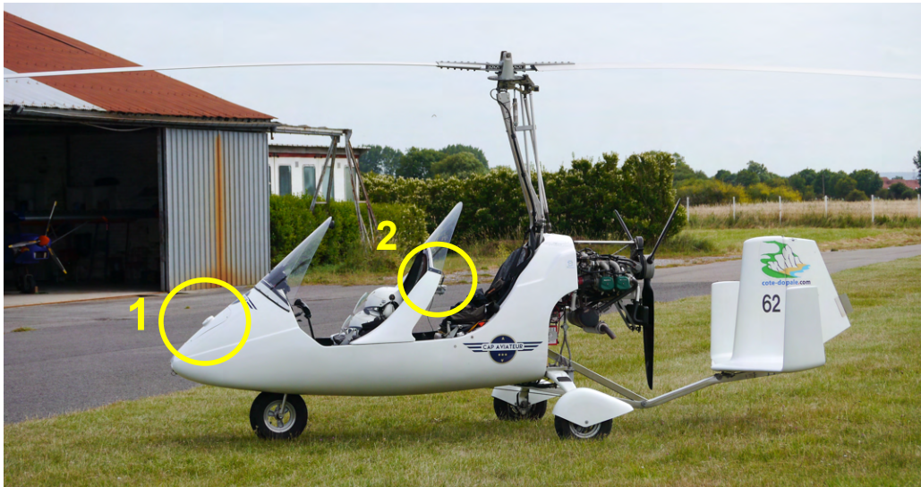
Figure 3.3: Aircraft used in the experiment. (1) GNSS - R antenna, (2) Extra GPS antenna + INS for flight control purposes.
